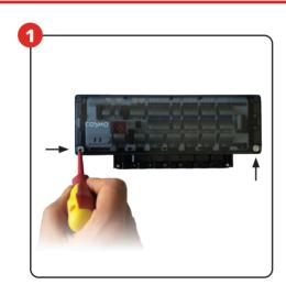
Remove the top cover of the control box
