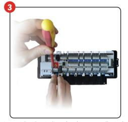
Connect the wires to the spring clamps according to the wiring diagrams. You can run the wires in the tunnel under control box housing.
