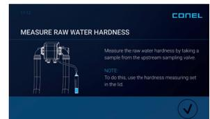
Measure and check the soft water hardness.
