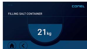
The amount of salt in kg is calculated automatically by an ultrasonic sensor. It cannot be set manually.
