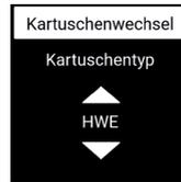
2. Use the  $\blacktriangle$  or  $\blacktriangledown$ -button to determine the cartridge type (HWE, HVE or HVE+).
