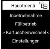
Press the  $\checkmark$ -button to start changing the cartridge.
