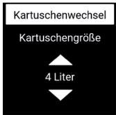
3. Use the  $\blacktriangle$  or  $\blacktriangledown$ -button to select the size of the cartridge (2.5, 4 or 7 litres).
