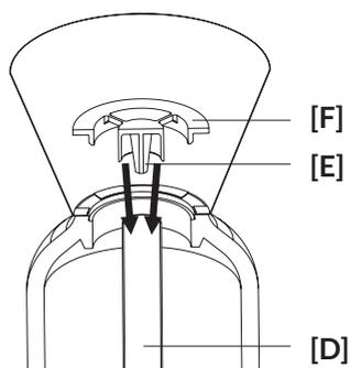
Now fill the corresponding resin through the funnel into the cartridge.
