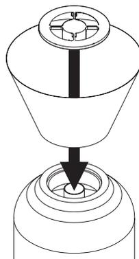
Place the funnel on the opening of the cartridge and center the lance [D] in the cartridge with the thorn [E] of the centering disk [F].
