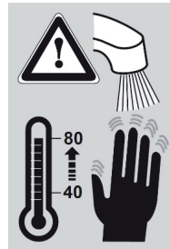
No temperature-stop fitted gives full hot supply temperature, upwards of 65°C. NOT RECOMMENDED!
