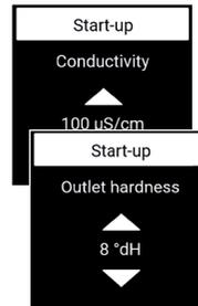
4. Use the  $\blacktriangle$  or  $\blacktriangledown$ -button to set the desired conductance (only possible with demineralisation) or the initial hardness (only possible with softening).
