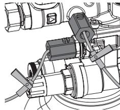
**6.** Mount the two needle valves of the meter to the maintenance ball valves.
