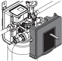
**1.** Pull off the insulation shell off.
