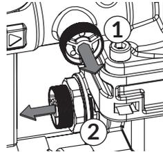
**4.** Remove the plug of the inlet (1) and intermediate pressure chambers (2).
