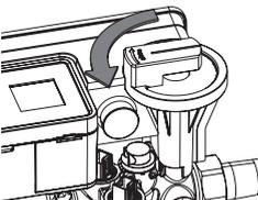
**7.** Mount the meter and open the shut-off valve on the outlet side.
