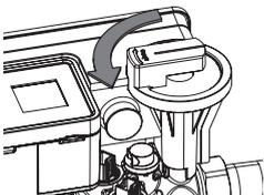
**5.** Open the shut-off valve on the output side.
