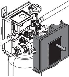
**1.** Pull off the insulation shell off.
