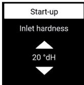
3. Use the  $\blacktriangle$  or  $\blacktriangledown$ -to set the measured input hardness.
