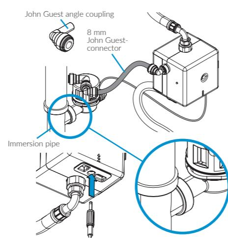
To cover several installation options, the Siphon Connection Set includes a second flexible hose to connect the connection valve with the HYGIENE BOX CONEL under consideration of the actual installation situation.
