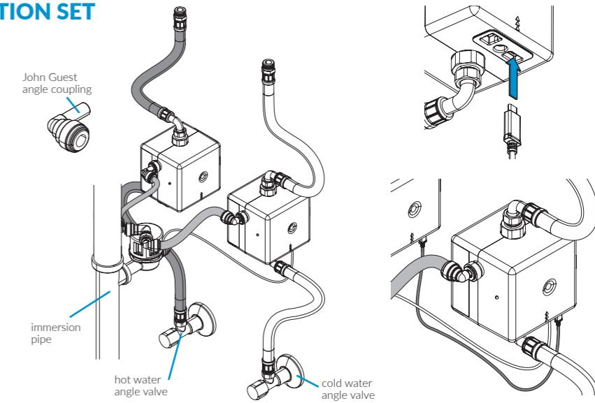
Make sure the drain hose slopes towards the tundish!
